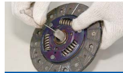
③ Apply the Grease to Spline Hub Teeth
