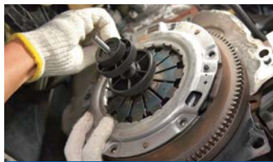
⑦ Installing to Fly Wheel
