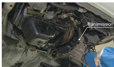
⑩ Reinstalling the Transmission
